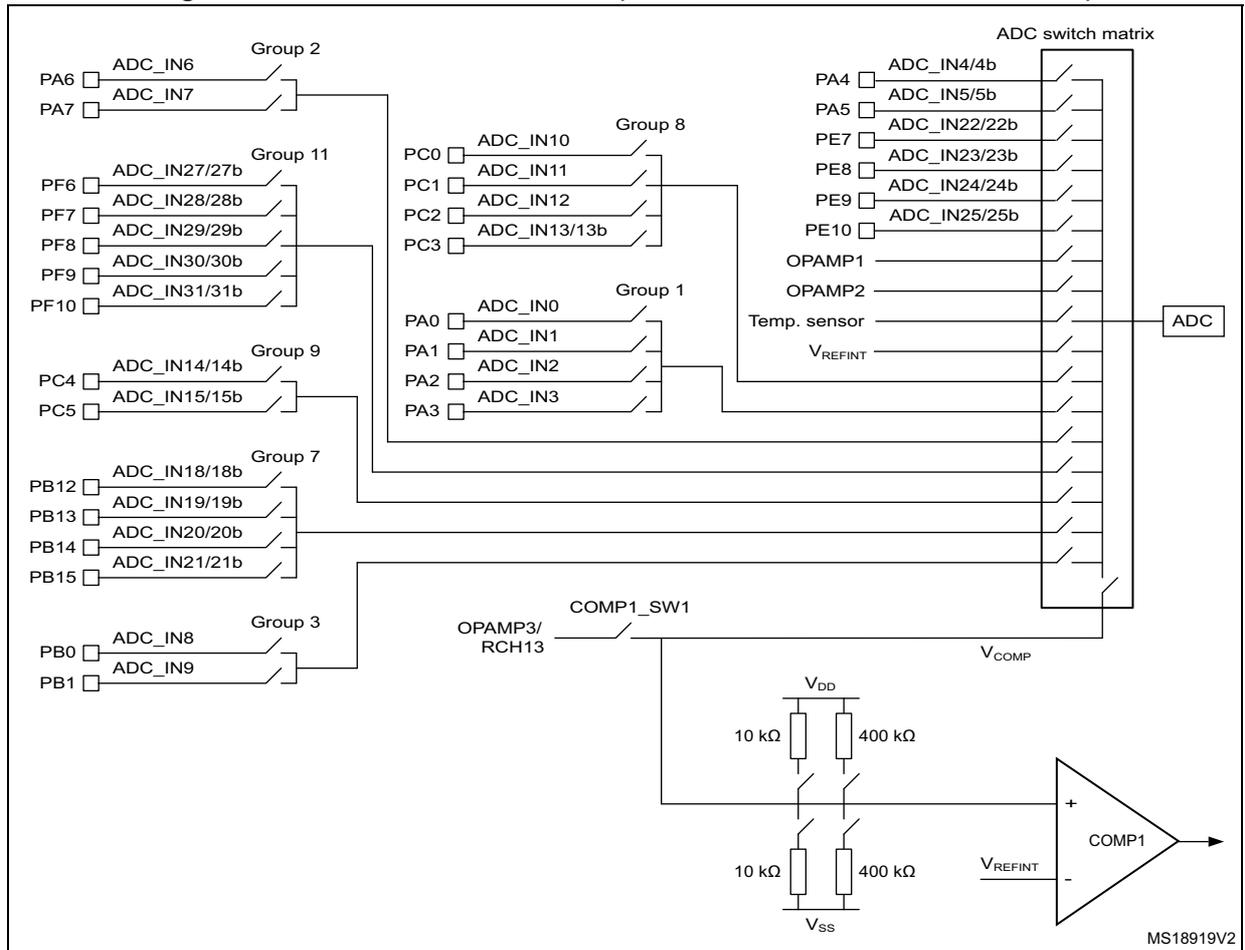
**Note:** *The internal reference voltage and temperature sensor cannot be used as COMP1 non-inverting input.*
