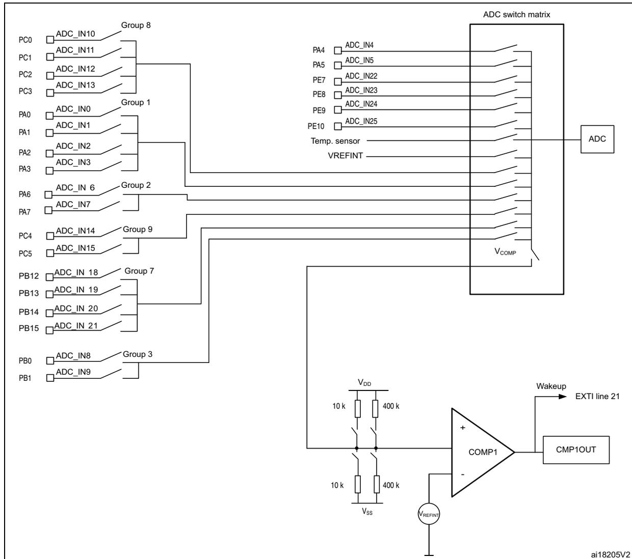
**Note:** The internal reference voltage and temperature sensor cannot be used as COMP1 non-inverting input.
