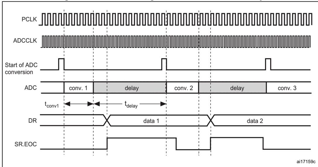
1.  $t_{conv1}$ : including sampling and conversion times (for instance 16 ADC clock cycles with the minimum sampling time)
