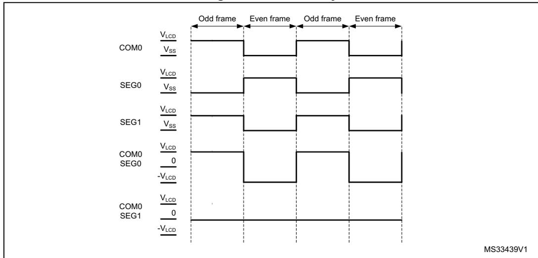
In each frame there is only one phase, this is why  $f_{frame}$  is equal to  $f_{LCD}$ . If 1/4 duty is selected there are four phases in a frame in which COM[0] is active during phase 0, COM[1] is active during phase 1, COM[2] is active during phase 2, and COM[3] is active during phase 3.
