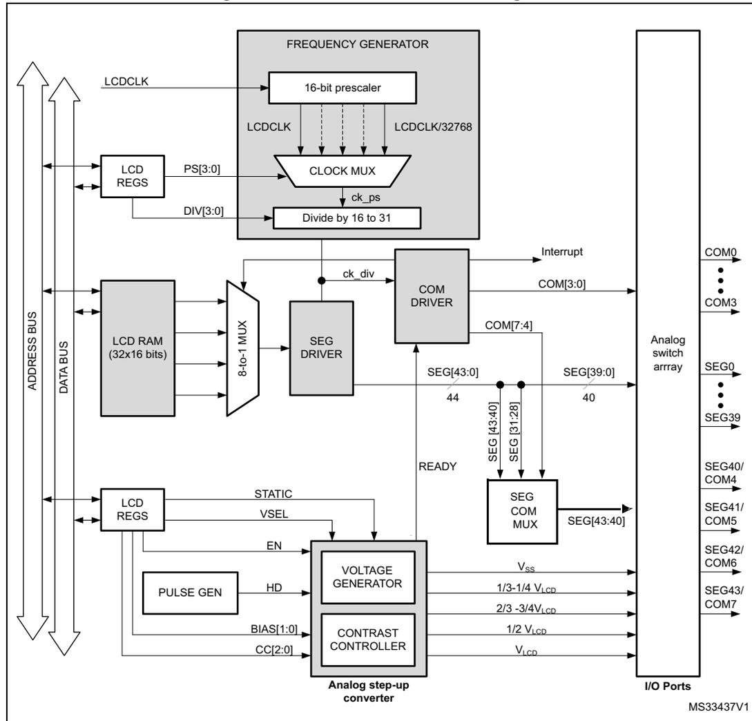
Note: LCDCLK is the same as RTCCLK. Please refer to the RTC/LCD clock description in the RCC section of this manual.
