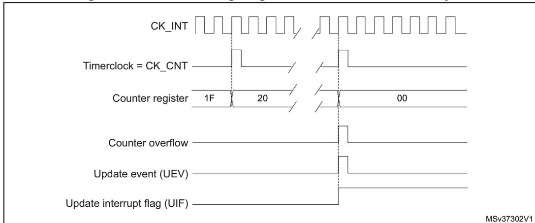
Figure 91. Counter timing diagram, Update event when ARPE=0 (TIMx\_ARR not preloaded)
