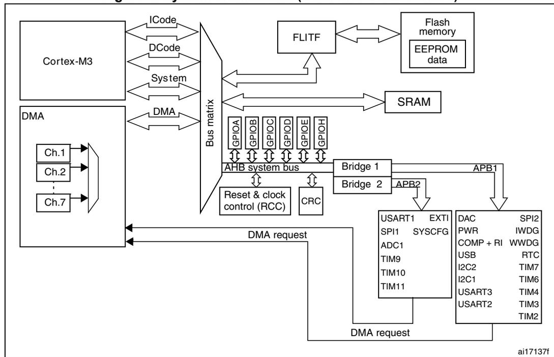
Figure 2. System architecture (Cat.3 devices)
