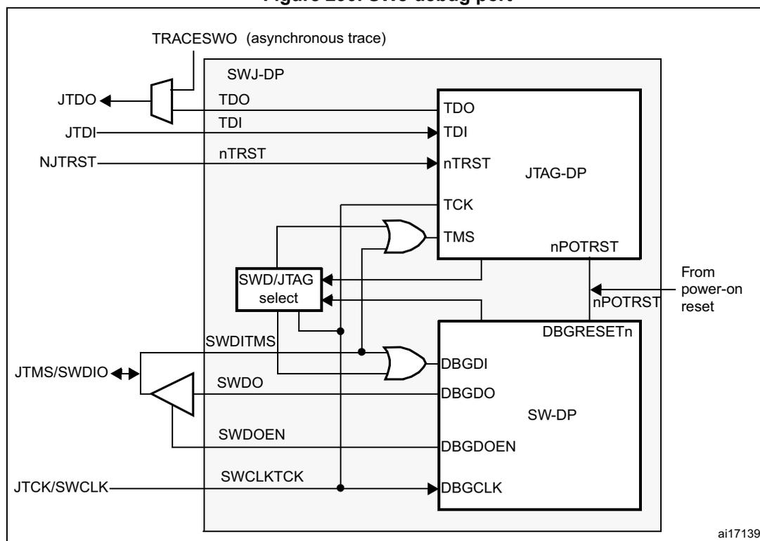
Figure 290 shows that the asynchronous TRACE output (TRACESWO) is multiplexed with TDO. This means that the asynchronous trace can only be used with SW-DP, not JTAG-DP.
