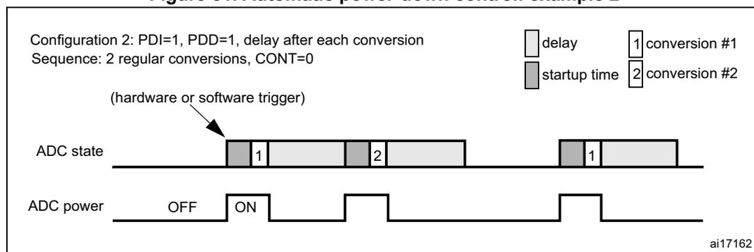
Figure 52. Automatic power-down control: example 3
