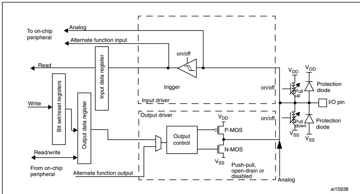
Figure 19. Basic structure of a five-volt tolerant I/O port bit
