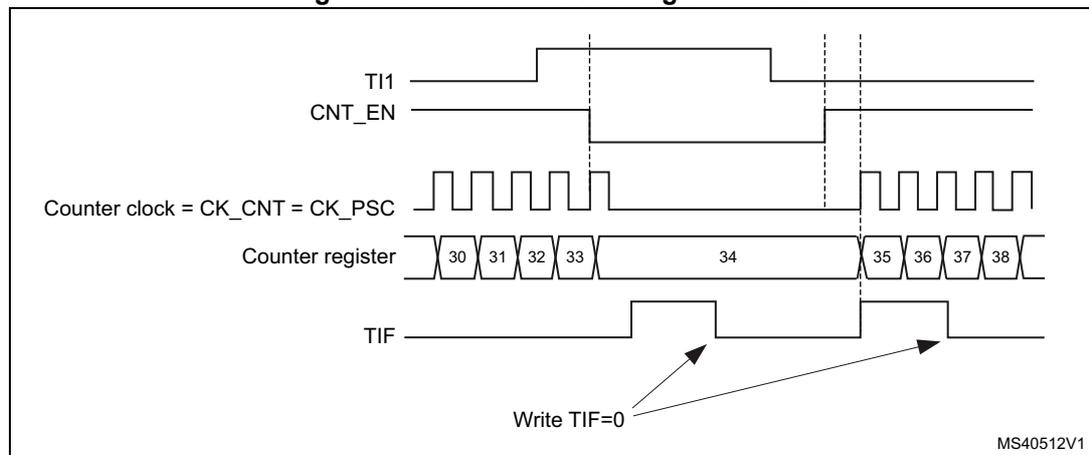
**Note:** The configuration “ $CCxP=CCxNP=1$ ” (detection of both rising and falling edges) does not have any effect in gated mode because gated mode acts on a level and not on an edge.
