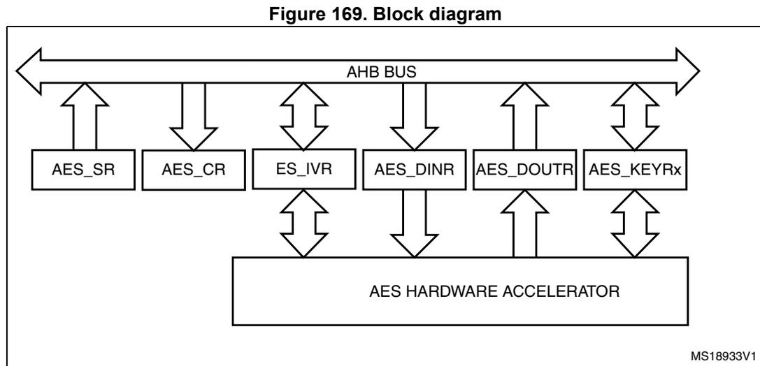
The AES accelerator processes data blocks of 128-bits (4 words) using a key with a length of 128 bits, and an initialization vector when CBC or CTR chaining mode is selected.
