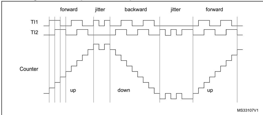
Figure 119 gives an example of counter behavior when TI1FP1 polarity is inverted (same configuration as above except CC1P=1).
