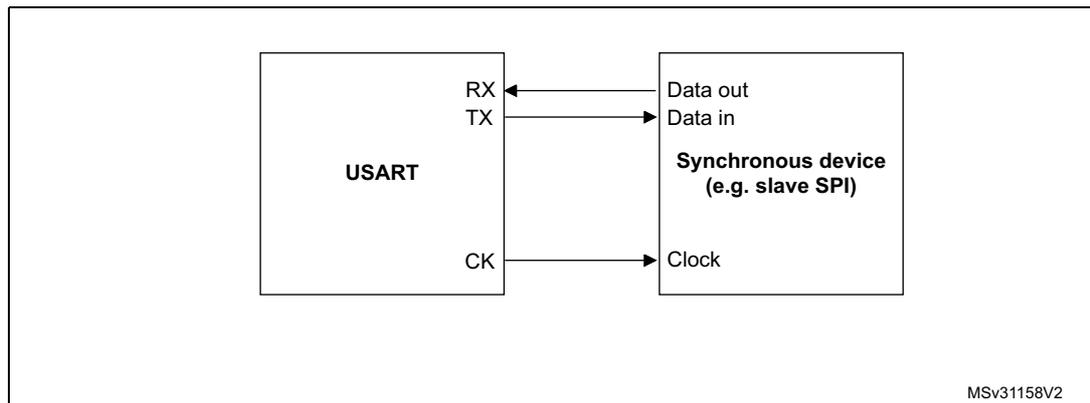
Figure 227. USART data clock timing diagram (M=0)
