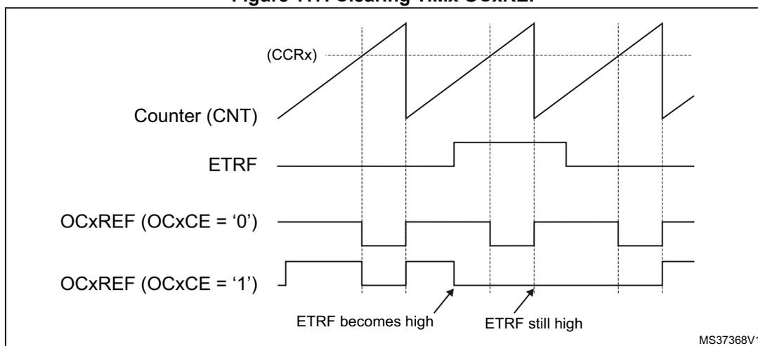
Note: In case of a PWM with a 100% duty cycle (if  $CCR_x > ARR$ ), OCxREF is enabled again at the next counter overflow.
