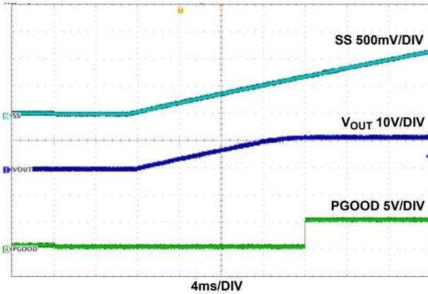
FIGURE 26. TRACKING;  $V_{IN} = 48V$ , LOAD = 0A, MODE = CCM
