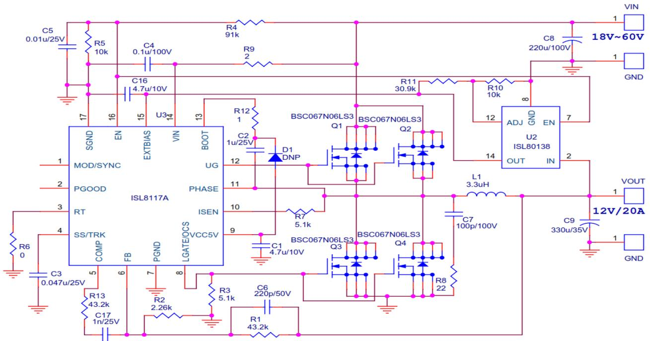
FIGURE 4. ISL8117A EVAL12Z EVALUATION BOARD SCHEMATIC
