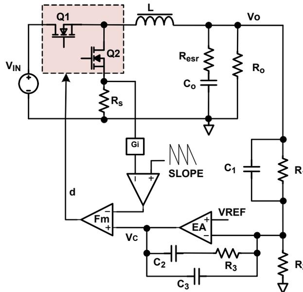
FIGURE 32. VALLEY CURRENT MODE BUCK CONVERTER CIRCUIT
