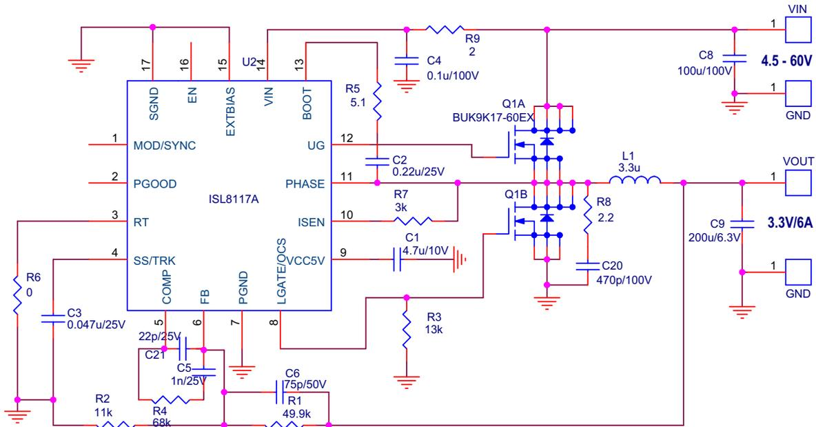
FIGURE 5. ISL8117A EVAL22Z EVALUATION BOARD SCHEMATIC
