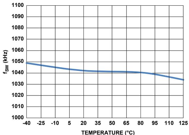
FIGURE 10. SWITCHING FREQUENCY vs TEMPERATURE ( $R_T = 36k\Omega$ )
