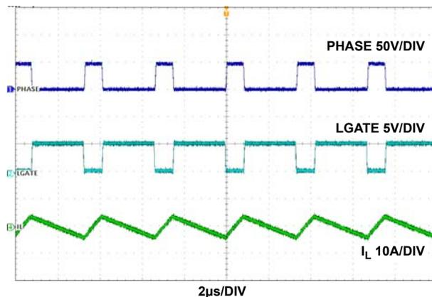
FIGURE 19. PHASE, LGATE, AND INDUCTOR CURRENT WAVEFORMS
