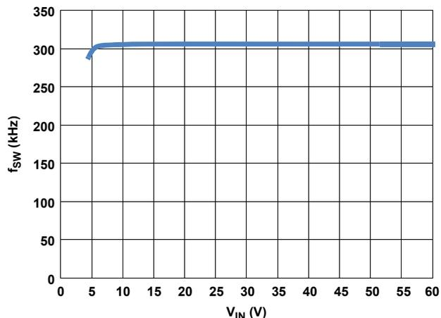
FIGURE 11. SWITCHING FREQUENCY vs  $V_{IN}$
