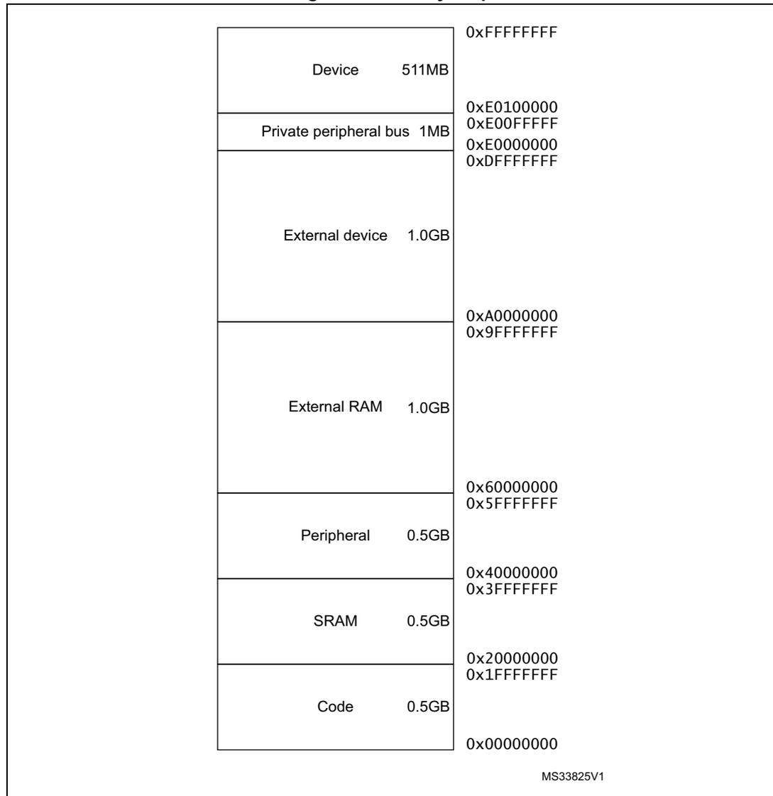
The processor reserves regions of the *Private Peripheral Bus* (PPB) address range for core peripheral registers, see [1.3: About the STM32L0 Cortex-M0+ processor and core peripherals on page 9](#).
