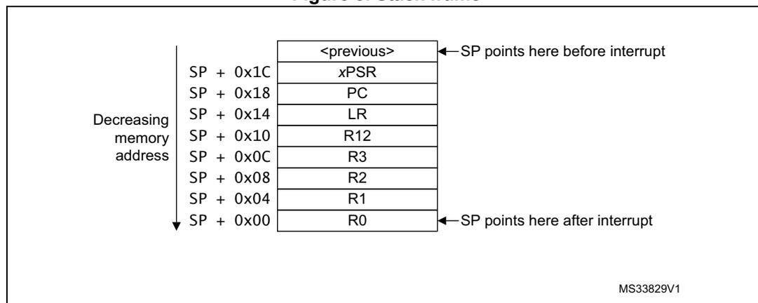
Immediately after stacking, the stack pointer indicates the lowest address in the stack frame. The stack frame is aligned to a double-word address.
