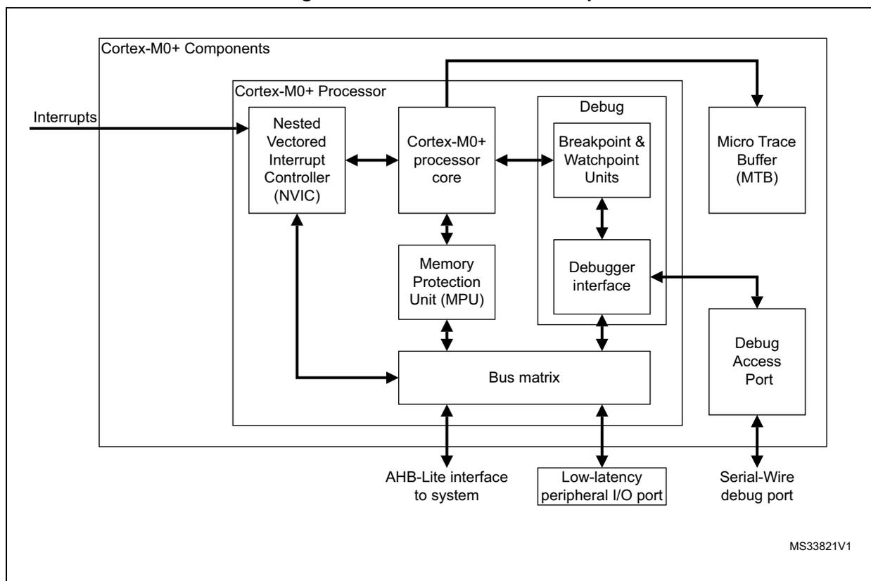
The STM32L0 Cortex-M0+ processor is built on a highly area and power optimized 32-bit processor core, with a 2-stage pipeline Von Neumann architecture. The processor delivers exceptional energy efficiency through a small but powerful instruction set and extensively optimized design, providing high-end processing hardware including a single-cycle multiplier.
